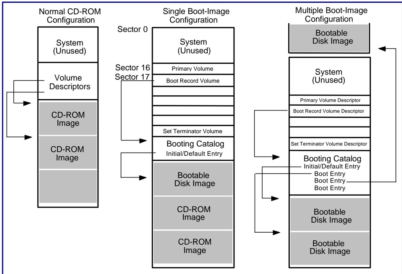
Figure 1. Three types of CD-ROM configuration:
